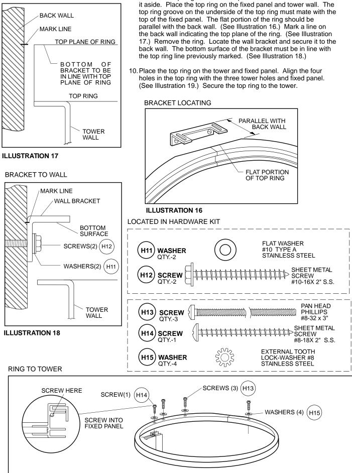
9. Locate the top ring. Remove the plastic retainer extrusion and set
